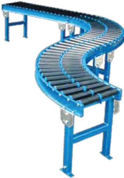
Gravity Roller conveyor is normally used where the cost of powered conveyor is generally unjustifiable and where the use of free gravity forces will allow the product to move freely along the conveyor.
