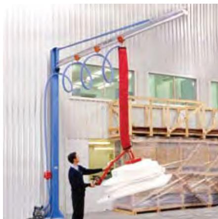
Jib Crane with Vacuum Lift attachment
